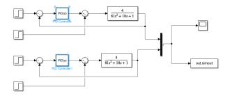
Figure 13: Simulink Model with 5 disturbance at 70s
