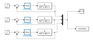
Figure 10: Simulink Model for PI controller
