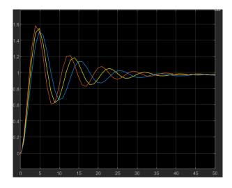
Figure 9: Simulink Result of P Controllers
