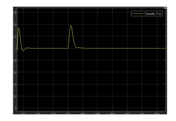
Figure 16: Simulink Result with 2 disturbance at 70s and 140s
