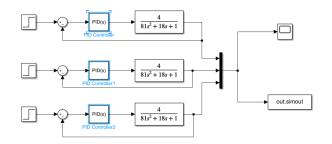
Figure 8: Simulink Model of P Controllers
