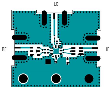
Figure 10. HF/VHF/UHF Evaluation Board Layout (DC933A)
