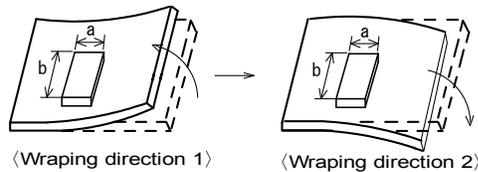
Products(wrapping direction 1, wrapping direction 2) shall be located carefully so that products are not subjected to the mechanical stress due to warping the board. Because they may be subjected the mechanical stress in order of wrapping direction 1>wrapping direction 2.
