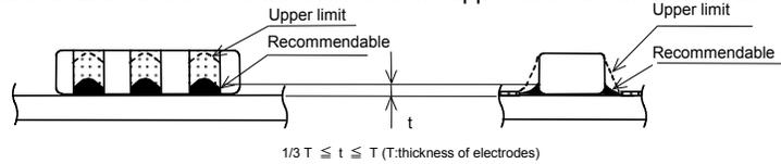
Accordingly increasing the solder volume, the mechanical stress to Chip is also increased. Exceeding solder volume may cause the failure of mechanical or electrical performance.
